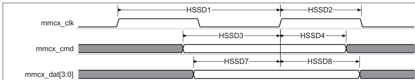
Figure 6-65. MMC/SD/SDIO – High-Speed SD Mode – Data/Command Receive
